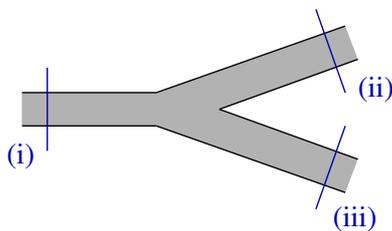
Consider a waveguide junction that connects single-mode open (!) dielectric channels in a y-shaped, symmetric (central horizontal plane) structure, The junction is supposed to be sufficiently long (“adiabatic”), such that reflections (here in the “common” meaning, including any transmittances (ii)  $\leftrightarrow$  (iii)) can be neglected. All media are reciprocal.
