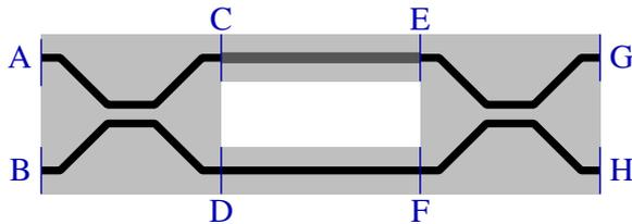
A circuit consisting of two couplers, connected by two (decoupled) segments of not-necessarily identical waveguides, constitutes a variant of a Mach-Zehnder-interferometer (MZI).
