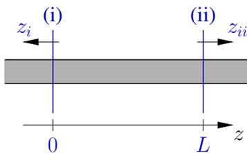
Consider a segment of length  $L$  of a straight lossless dielectric waveguide, made from linear isotropic material. Assume that the waveguide supports two guided modes with propagation constants  $\beta_1, \beta_2$ . Obviously, reflections do not occur, and the “circuit” is reciprocal.
