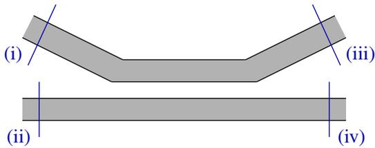
Consider a directional coupler that connects single-mode dielectric channels. The structure is symmetric with respect to the central vertical plane (figure), but not, at first, with respect to any horizontal plane.
